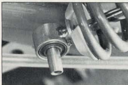
Nifty innovation; barrel shaped shock bushings do the same job as a heim joint, with less complications.
