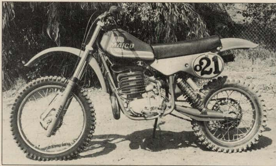
Totally changed for '81, the new 490 Maico is long and lean. Obvious changes on the new big bore are piggyback Corte & Cosso shocks, fresh plastic and a dramatically lengthened wheelbase.
