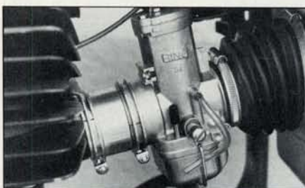
Flaw in an otherwise sound design: the aluminum inlet tract let grit and crud pass through. The Bing carbureted well, once we dialed the jetting in.
